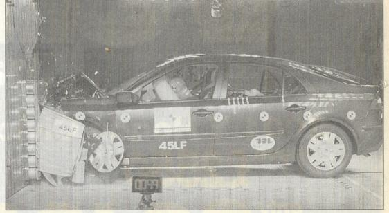
(Euro NCAP). Standard vehicles are bought randomly and anonymously from dealers for these tests, ensuring that none have been specially modified.
